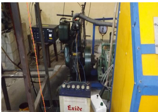
Fig1.1 Experimental setup of GHSI LHR Engine Test rig
